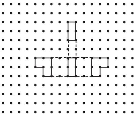
5. The following object is rotated  $270^\circ$  counterclockwise about the horizontal axis. Draw the front, top, and side views after the rotation is applied.
