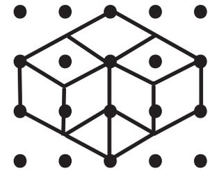
Draw the views of rotated objects using the same method you applied before. However, in this situation, first determine the new orientation of the rotated object. Then begin making your drawings.
